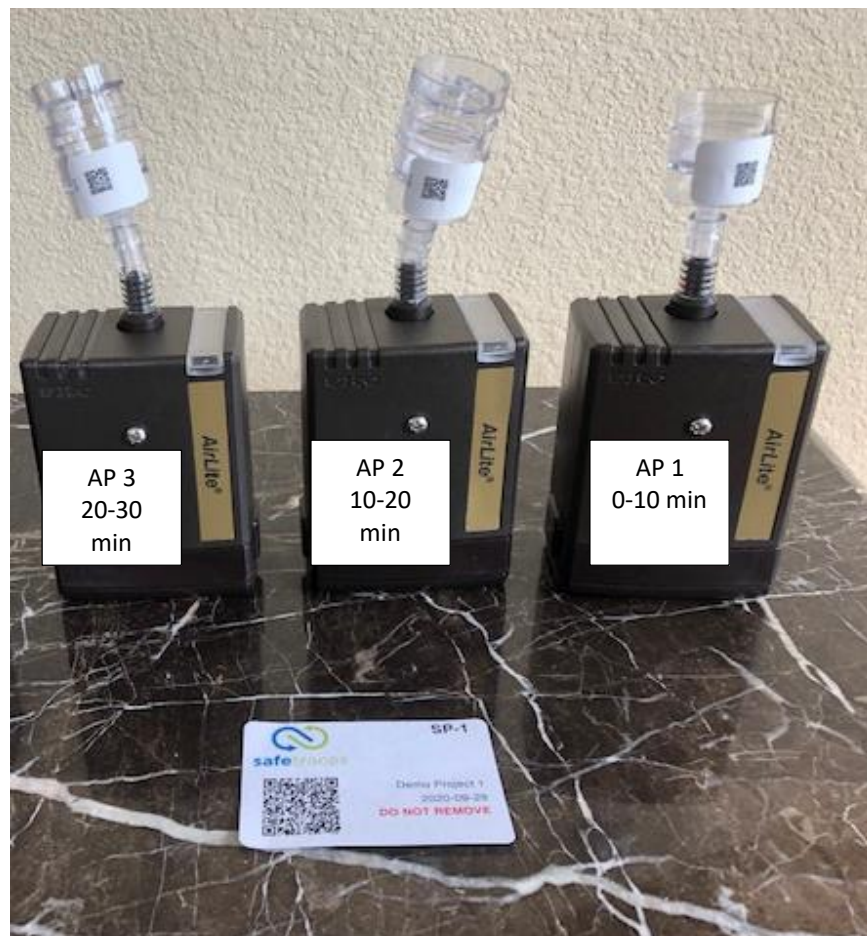
Sample Point Set-Up Note: Air Pump 1 (0-10 min) does not have a Cassette Top. Cassette Tops are on Air Pump 2 (10-20 min) and Air Pump 3 (20-30 min)
