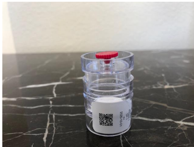
Plug the top cap with the Red Plug and bottom with the Blue Plug
